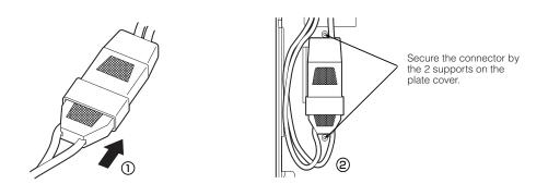
If you cannot secure the connector to the plate cover, the connector is not inserted completely.
